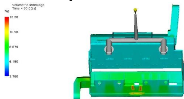
Fig. 8. Volumetric shrinkage of the part.
